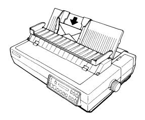
If it is necessary to eject the printed envelope, press the **ON LINE** button to set the printer off line. Then press the **LOAD/EJECT** button.
